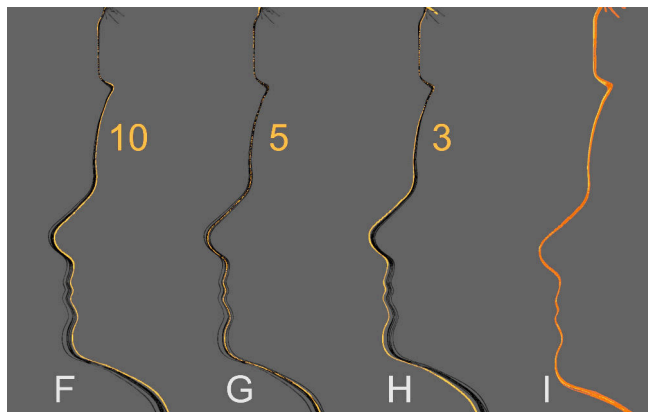
Figure2.8: F) Section view with all 8 models and the one with 10 small targets selected in orange. G) Selection of the model with 5 small targets. H) Selection of the model with only 3 targets. I) Manual rotation adjustment showing structural compatibility among all 8 models.
